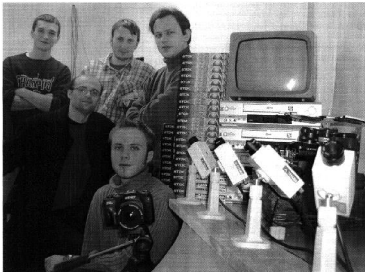
Figure 1 – Polish Automated Video Observations of meteors (PAVO) setup: four TAYAMA low light CCTV cameras called PAVO1, PAVO2, PAVO3 and PAVO4, four LG LV2798 VCRs, one old TV set for monitoring the video signal and a lot of TDK HS 240 video tapes. The rotating shutter for photographic observations is visible behind the cameras. Also in picture are (from left) on top: Konrad Szaruga, Piotr Kędzierski, Arkadiusz Olech; bottom: Mariusz Wiśniewski and Andrzej Skoczewski. The picture was taken after observation of the Leonid shower maximum. ,
