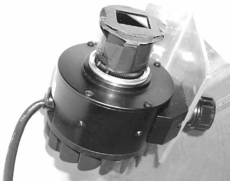
Figure 1: The MicroTelescope (MiT): CCD Camera, 4.5 mm lens and I filter.
